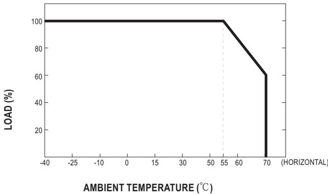
Note : At high ambient temperature  $T_a=70^{\circ}\text{C}$ , if HLG-600H operates in C.C mode, the maximal current must not be greater than 60% of the rated current.
