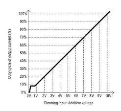
O Applying additive 10V PWM signal (frequency range 300~3KHz):
