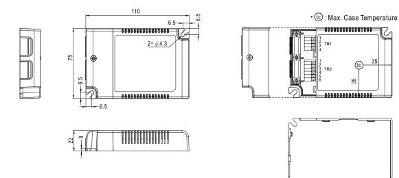
NOTE: Please use wires with a cross section of 0.75~1.5mm² for TB1 and wires with a cross section of 0.5~1.5mm² for TB2.
