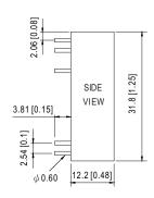
NOTE: Pin tolerance ±0.05mm
