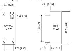
NOTE: Pin tolerance ±0.05mm
